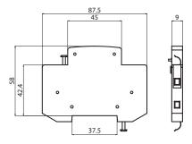
The PS EFI is fixed to EFI series switches. The width of the device is 9 mm, other dimensions are in compliance with EFI switches. The auxiliary switch PS EFI is used for the remote signalling of the state of contact's condition (closed/open) of EFI switches. During fitting, the EFI must be switched off. PS EFI and DA EFI can not be mounted both together, because both can only be mounted on the right side of EFI.
