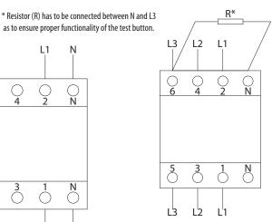
RCD ETI Type B in 3-phase system without neutral conductor - U<sub>n</sub>=400V 30mA: R=2k7/1W (500V)
