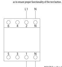
RCD ETI Type B in 1-phase system  $U_n = 230V$
